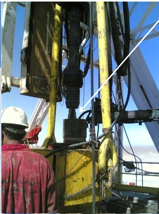
Fill up tool while filling casing with mud
