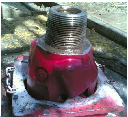
12.25" Bit (Reed Hycalog) in Bit breaker
