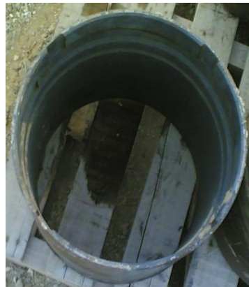
Wear bushing: Installed in B.H. by test plug during running with 12.25" drilling assembly
