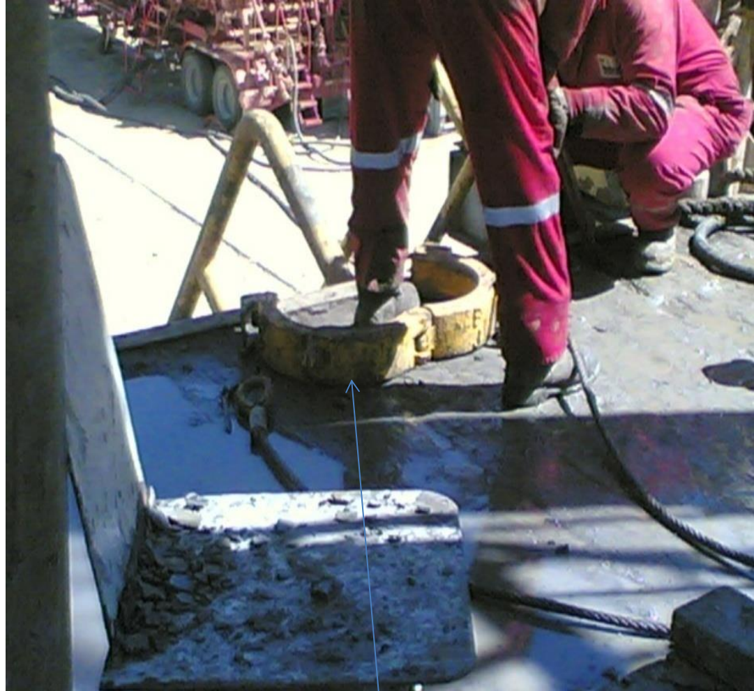
Single elevator to elevate casing from cat walk then through V-door to be above well
