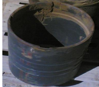
Wear bushing: Installed in B.H. by test plug during running with 12.25" drilling assembly
