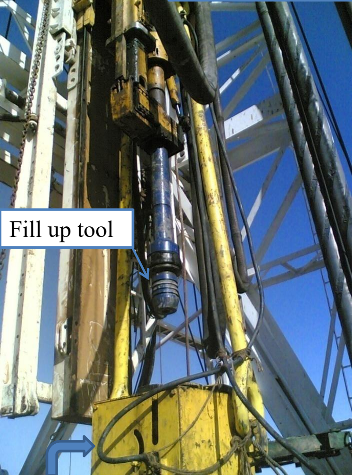
Spider slips to engage casing while running in hole at high depths (engage high weights)
