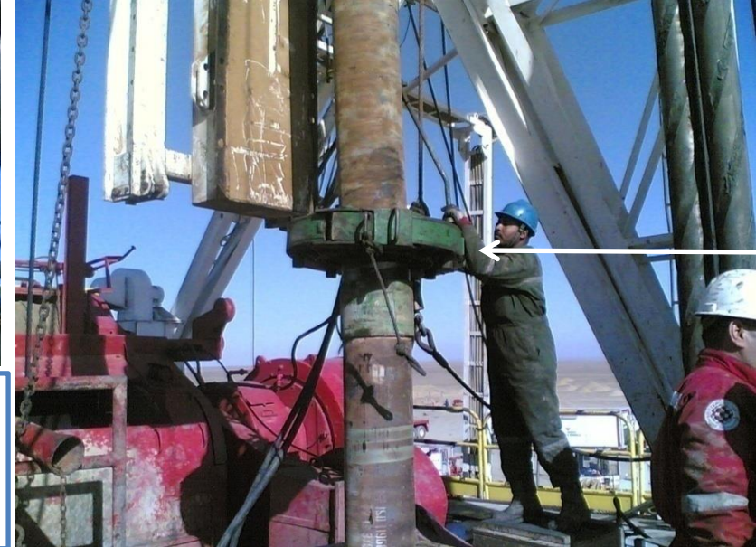
Power tong: screw casing till had its torque
