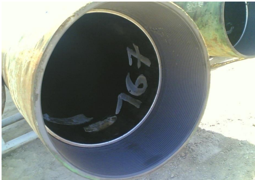
B-Profile gauge: Check thread by stamp
