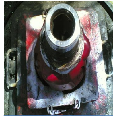
12.25" Bit (Reed Hycalog) in Bit breaker
