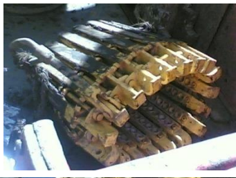
Casing slips to engage casing while running in hole
